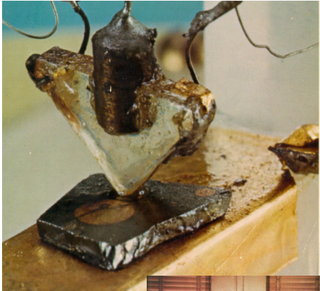
1º Transistor, 1947 Bell Labs: Bardeen, Brattain, e Shockley
